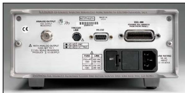
Figure 7. Model 2182A rear panel
