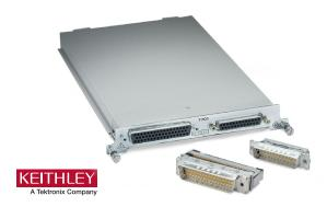
The 7701 plug-in module offers 32 channels of 2-pole or 16 channels of 4-pole multiplexer switching. Its 32 channels can be configured for common-side 4-wire ohms. They can also be configured as two independent banks of multiplexers. It is ideal for RTD or thermistor temperature applications.
