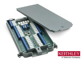
The 7702 plug-in module offers 40 channels of 2-pole or 20 channels of 4-pole multiplexer switching that can be configured as two independent banks of multiplexers. The 7702 provides two additional protected channels for current measurements. It is ideal for RTD, thermistor, and thermocouple temperature applications.
