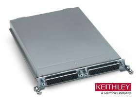
The 7703 plug-in module offers 32 channels of 2-pole or 16 channels of 4-pole multiplexer switching that can be configured as two independent banks of multiplexers. The non-latching reed relays provide high speeds and are designed for 300 volt, 500 mA; 10 VA. The relay closures are stored in onboard memory. The 7703 is ideal for RTD and thermistor temperature applications.
