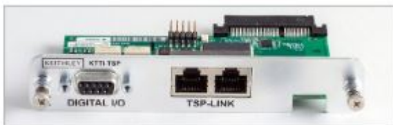
KTTI-TSP TSP-Link interface with 6 digital I/O ports.
