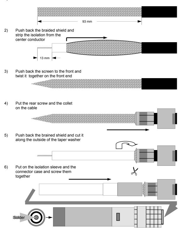
7) Solder the cable center conductor with the plug center contact
