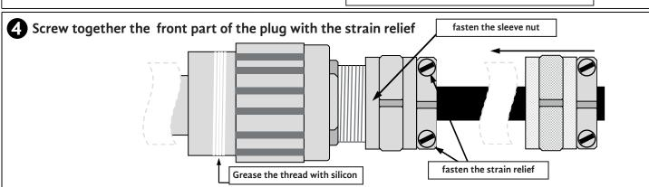
This mounting instruction is also valid logically for connectors of the same construction e.g. S130, HVS 65, HVS 100 or HVS 150. The difference is only in the length of the plug
