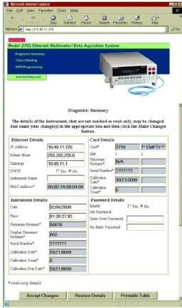
Built-in Web diagnostic tool (Model 2701 only) sends command strings and receives data over the network. It also reads and sets network parameters.
