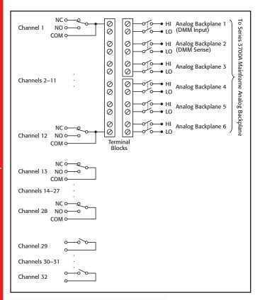
RELAY SWITCH CONFIGURATION: 32 general purpose independent channels. 28 channels of Form C switching at 2A and 4 channels of Form A switching at 7A. Relays can be connected to each other and backplane via removable terminal blocks.
