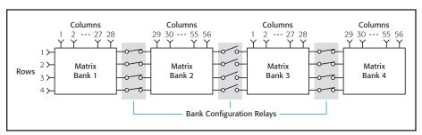
Dual 4×56 (1-wire) or single 4×56 (2-wire) matrix configuration using bank configuration relays
