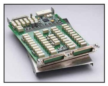
The Model 3721 offers two independent banks of  $1\times20$  two-pole multiplexers that are ideal for general purpose switching, including temperature measurements. The two banks can automatically be connected to the Series 3700A mainframe backplane and optional DMM through the analog backplane connection relays. This connection allows the mainframe to reconfigure the Model 3721 as a single  $1\times40$  two-pole multiplexer or to enable card-to-card expansion for even larger configurations.
