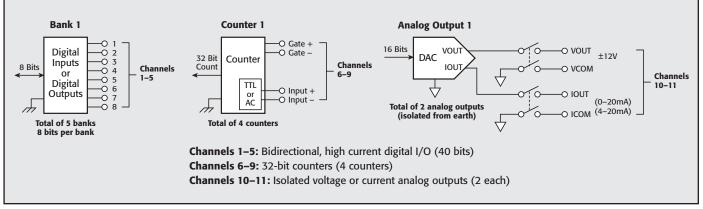
Figure 1. Block diagram
