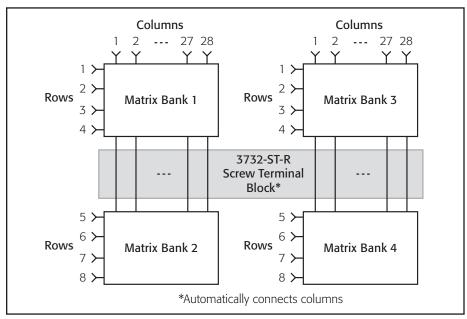
Dual  $8\times28$  (1-wire) or single  $8\times28$  (2-wire) matrix configuration using one Model 3732-ST-R screw terminal block
