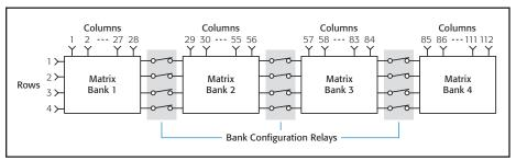
Single 4×112 (1-wire) matrix configuration using bank configuration relays
