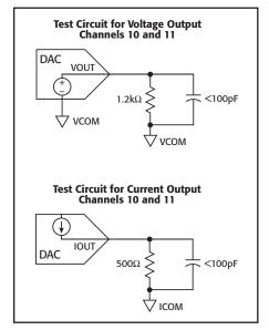
Figure 3. Standard load test circuits
