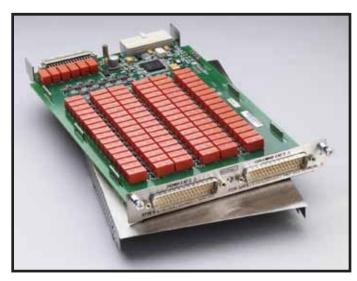
The Model 3730 is a two-pole, 6 row by 16 column matrix card. It can connect up to six differential instrument channels to any combination of 16 DUTs (devices under test). Any row can be connected to the Series 3700A mainframe backplane by using the analog backplane connection relays. This allows for easy matrix column expansion. A matrix of up to 6 rows by 96 columns can be supported within a single Model 3706A mainframe (with six Model 3730 cards).
