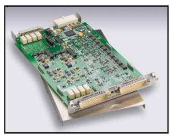
Use the Model 3750 to monitor and control your automated test system. The flexibility and speed provided by the 40 digital I/O bits, four counters, and two analog outputs make it well-suited for a wide variety of system control applications.
