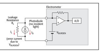
Figure 1. Dark Current Measurement with Burden Voltage Uncorrected
