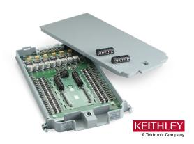
The 7710 plug-in module offers 20 channels of 2-pole or 10 channels of 4-pole relay input that can be configured as two independent banks of multiplexers. The relays are solid state, providing long life and low maintenance. Solid-state relays usually have 100 times longer life than mechanical relays. It is ideal for long-term data logging applications as well as for demanding high-speed applications.
