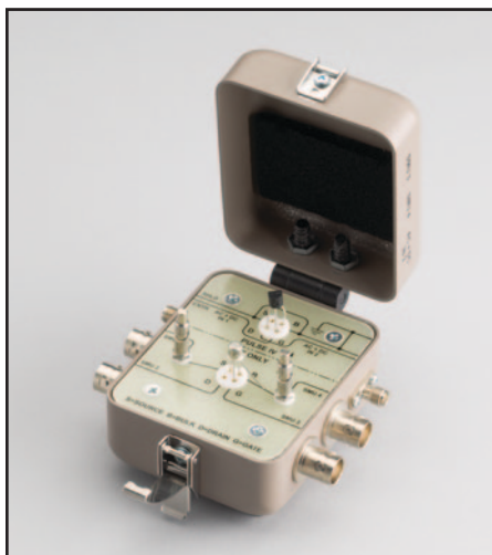
Model 8101-PIV: DC and pulse I-V demo fixture that is a metal case with four female triax connectors, two SMA connectors, and a latch. Inside the test fixture are two 4-pin device holders (transistor sockets) and two plungers for parts with two leads.
