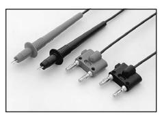
Model 5805 Kelvin Probes: 2 spring-loaded test probes, red and black, 0.9m (36 in) with banana plug termination. Designed to be used with Keithley instruments that measure 4-terminal resistance and in-circuit current. 1/8-in spacing between pin tips. A package of 8 replacement contacts (P/N CS-551) is available.
