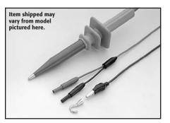
Model 1600A High Voltage Probe MAXIMUM INPUT: 40kV DC or peak AC to 300Hz. INPUT RESISTANCE:  $1000M\Omega$ . DIVISION RATIO: 1000:1 (into  $10M\Omega$ ).
