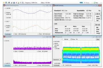
Analysis options for 802.11 standards are available. Here, an 802.11ac 80 MHz signal is analyzed, with displays of EVM vs. subcarrier number and symbol number, channel response vs subcarrier with a summary of WLAN measurements, and the DPX spectrum of the analyzed signal. An EVM of -44.26 dB and other signal measurements are seen in the summary panel.
