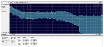
Phase noise and jitter measurements (Opt. 11) on the RSA5000 Series may reduce the cost of your measurements by reducing the need for a dedicated phase noise tester. Outstanding phase noise across the operating range provides margin for many applications. Here, phase noise on a 13 MHz carrier is measured at -119 dBc/Hz at 10 kHz offset. The instrument phase noise of < -134 dBc/Hz at this frequency provides ample measurement margin for the task.
