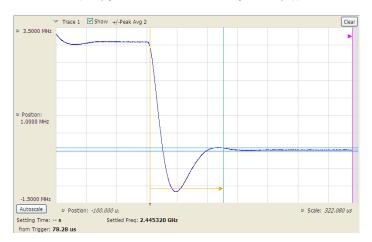
Settling time measurements (Opt. 12) are easy and automated. The user can select measurement bandwidth, tolerance bands, reference frequency (auto or manual), and establish up to 3 tolerance bands vs. time for Pass/Fail testing. Settling time may be referenced to external or internal trigger, and from the last settled frequency or phase. In the illustration, frequency settling time for a hopped oscillator is measured from an external trigger point from the device under test.
