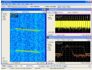
Once captured into memory, SignalVu provides detailed analysis in multiple domains. The spectrogram display (left panel) shows the frequency of an 800 MHz wide LFM pulse changing over time. By selecting the point in time in the spectrogram during the On time of the pulse, the chirp behavior can be seen as it sweeps from low to high (lower right panel).
