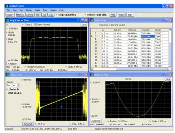
The Advanced Signal Analysis package (Option SVP) provides 27 individual measurements to automatically characterize long pulse trains. An 800 MHz wide LFM chirp centered at 18 GHz is seen here with measurements for pulses 7 through 18 (upper right). The shape of the pulse can be seen in the Amplitude vs Time plot shown in the upper left. Detailed views of pulse #8's frequency deviation and parabolic phase trajectory are shown in the lower two views.
